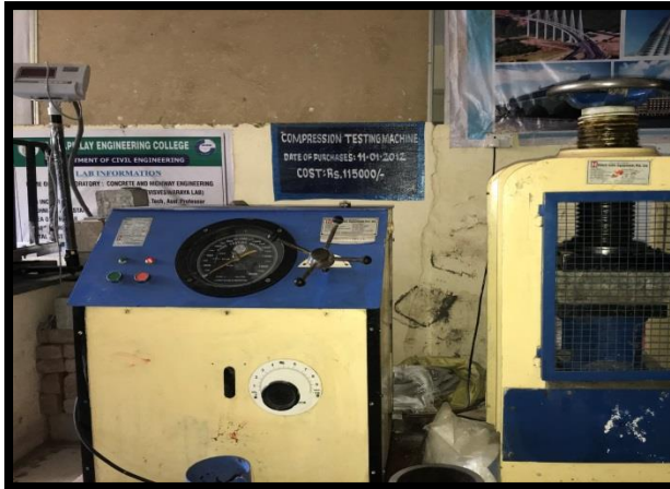
Fig: CTM machine for compressive strength of cubes
