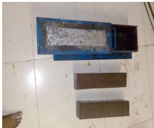
Fig:5.2 Casting for RC &FRC Beams
