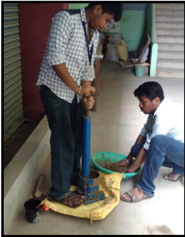
Fig: Soil compaction
