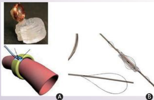
Fig.1. Implantable blood pressure sensor. (A) Surgically im- planted blood pressure sensor with a cuff-type design. The sensor is installed on the blood vessel directly. (B) Cardiomeems im- plantable blood pressure sensor.
