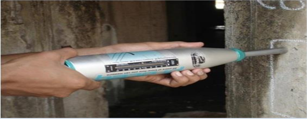
Figure: Rebound Hammer Test
