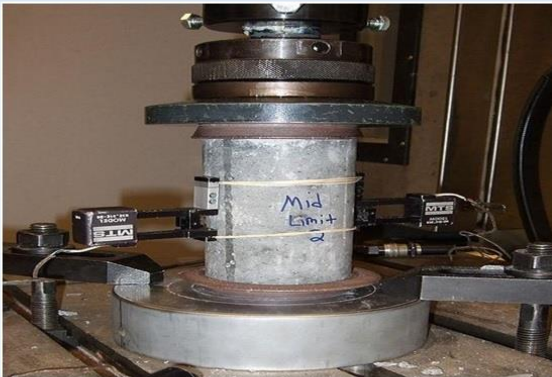
Figure: Compressive Test on Concrete
