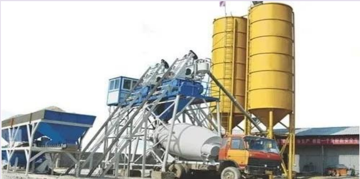
Ready Mix Concrete Batching Plant
